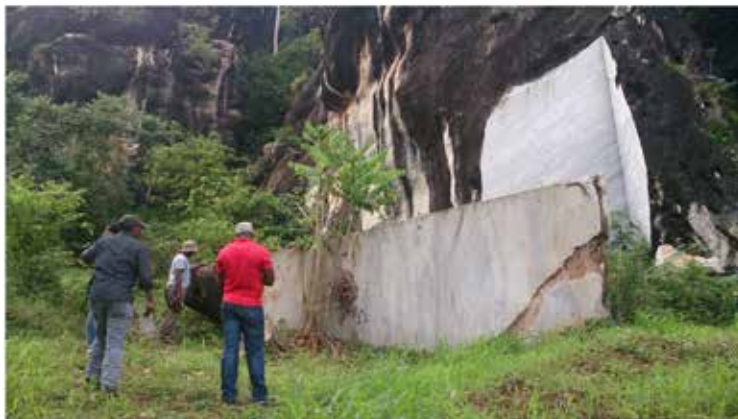
The outcrops seen: Metamorphosed dolomitic marbles observed in abandoned mine at Changa Village. The marbles are extensively distributed and well exposed in this area
